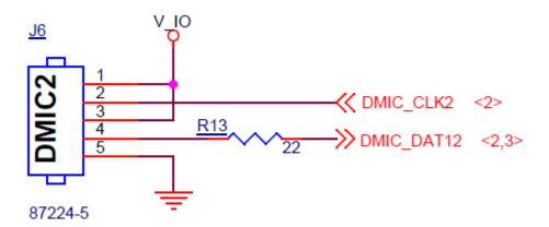
**Example DMIC Connector Signal Connections**
